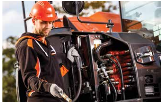
The excavator can be refuelled using an electric pump.
